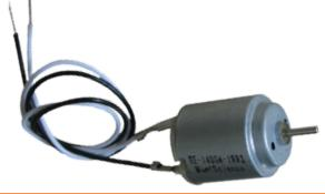
BHi torque DC motor with lead wires operates with 1.5 to 3.0 volts and runs at speeds of 2500 12% rpm. Dimensions are 40 mm L x 21 mm D. Weight 23g (0.8 oz). Exposed shaft of 8mm or more with option of strong magnets for more power.
